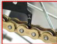
B. Lower the measuring nib. Extension rate will be shown on measuring nib where it touches the chain roller.
