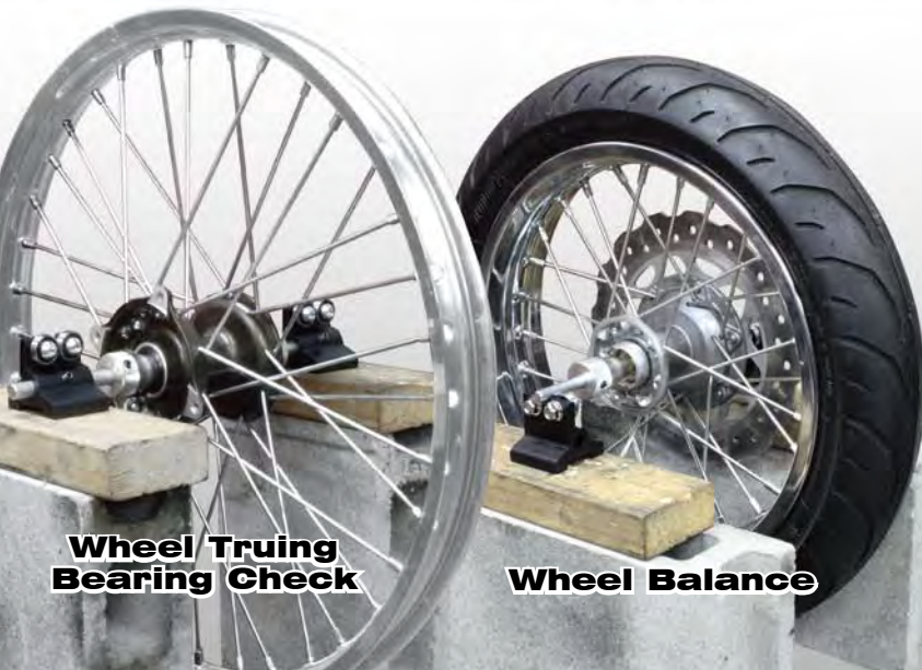
Lock wheel rod for wheel truing and bearing check.
